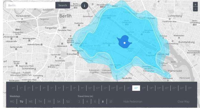
Figure 1: User interface with a) search bar, b) the main map with an Isoscope in Berlin, c) the 24 hours time selector, and d) additional buttons to select week day, travel time, and transport mode.
